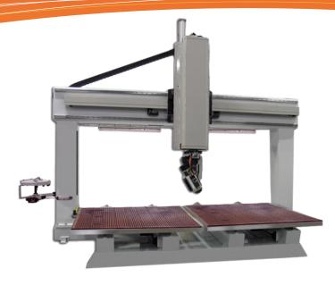
Mastermill SGF is a model designed for high-speed machining of nonferrous materials such as wood, polystyrene, resins, composites, aluminum, etc...
